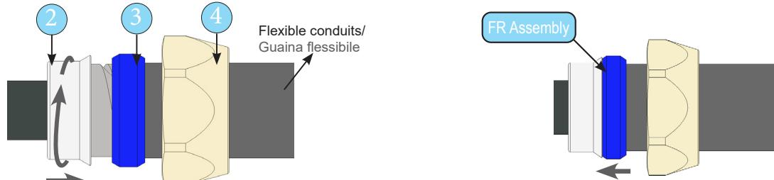
**Step 2** Insert part (1) inside the cable and hand tighten between body and nut (1 and 4).
